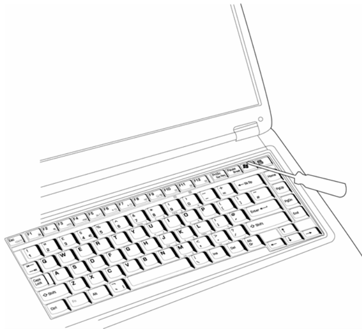
Figure 4-13 Removing the strip cover
